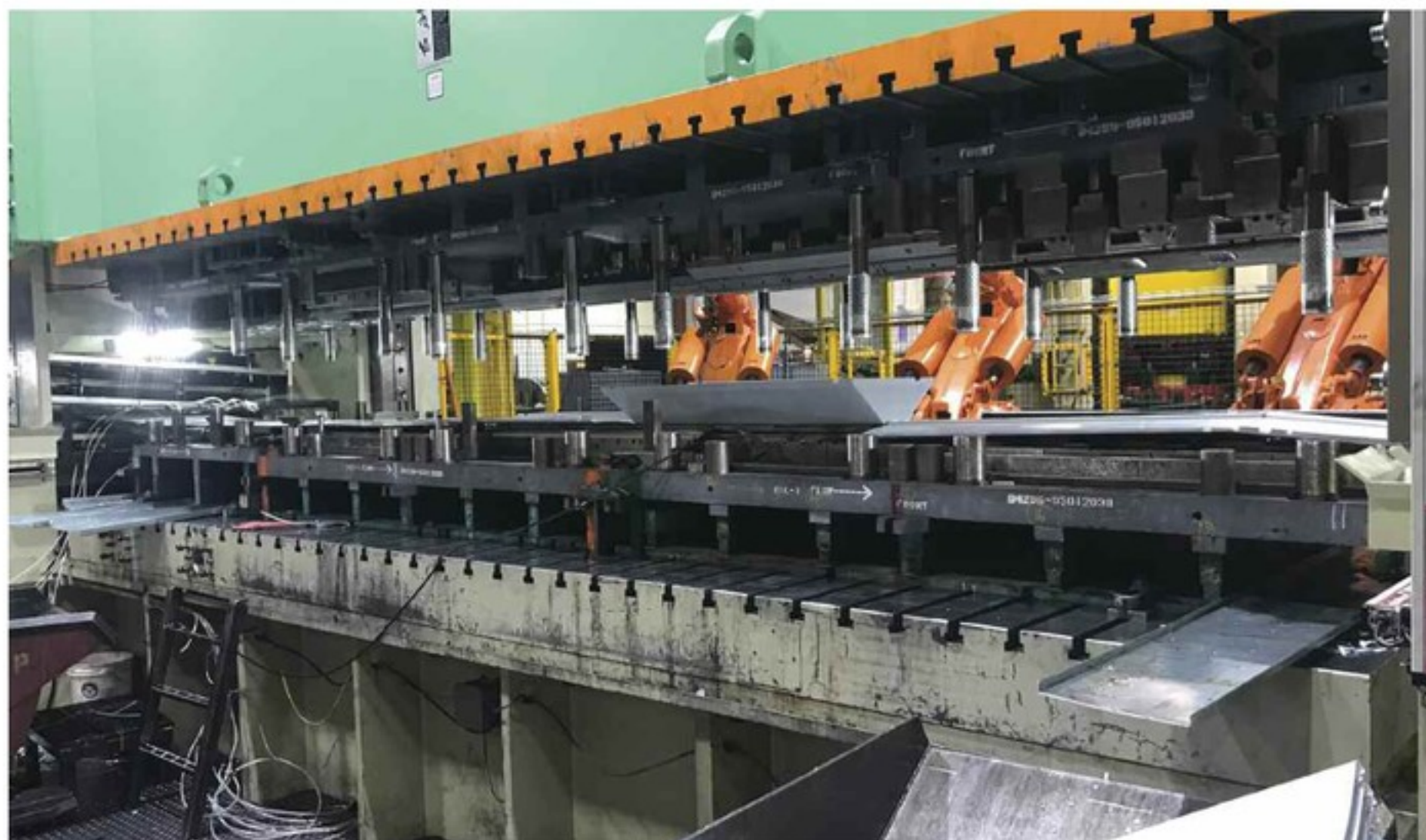
Lighting housings are shown being run on a progressive die.
