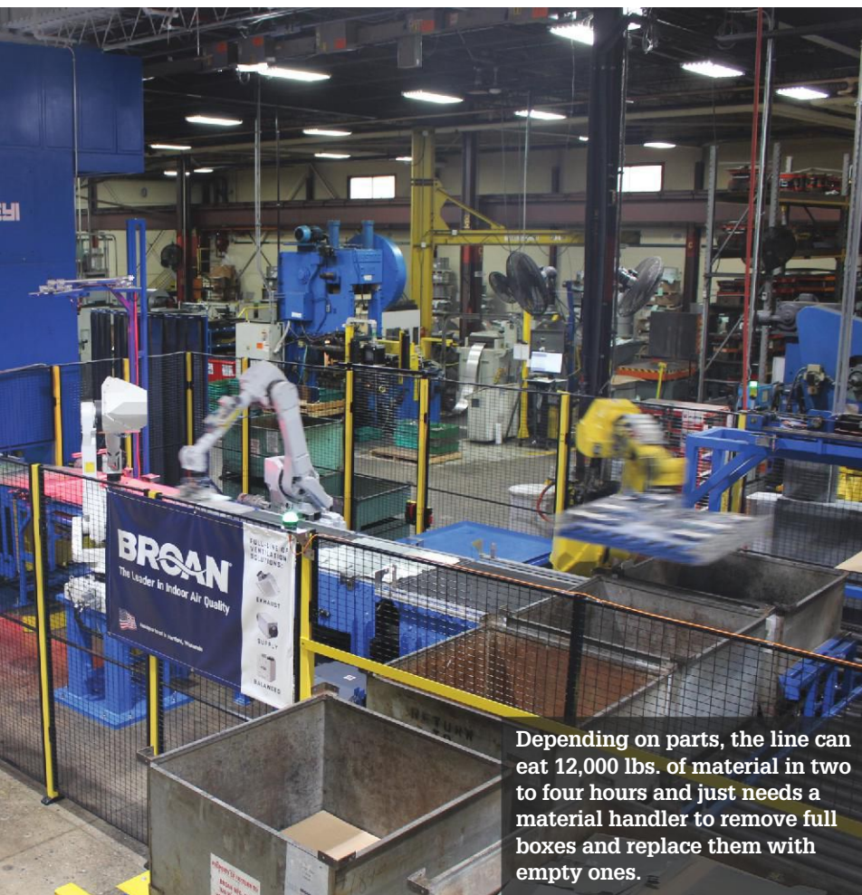
The third robot at the end of the line takes the pattern of parts and layers them in a gaylord bin for downstream operations.
